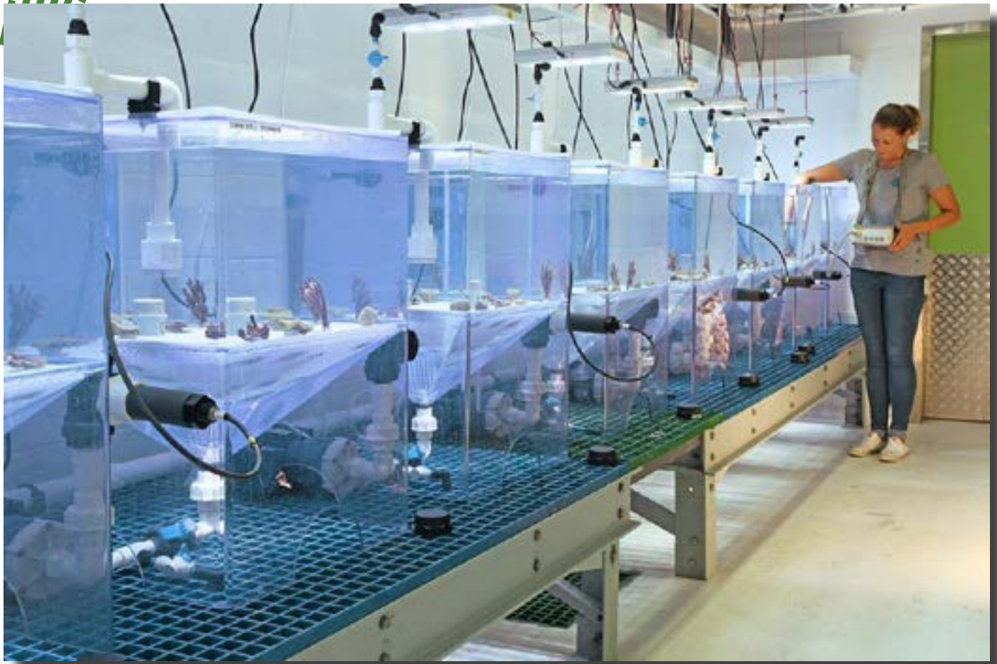
Dosing tanks that have been set up at UWA to test coral and sponge tolerance to sediment load.
