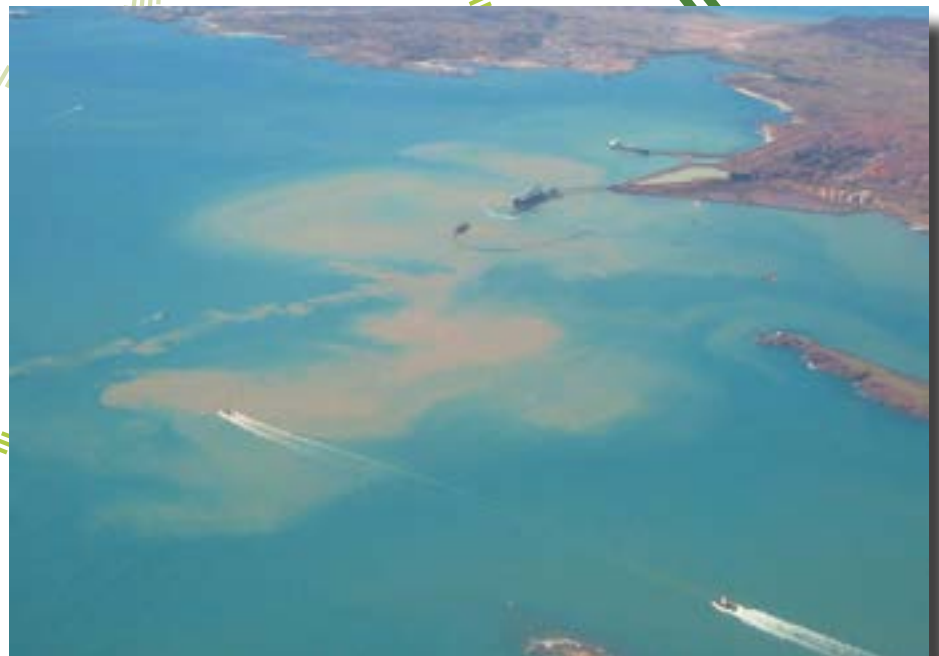
An aerial photo of dredging plumes created at Pt Parker on the Burrup Peninsula, Dampier.
